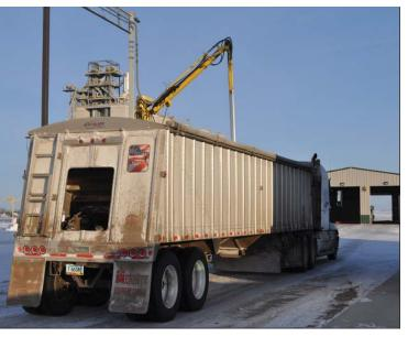
Inbound truckload of wheat is sampled as the truck sits on an inbound scale before being routed to one of two receiving pits.
